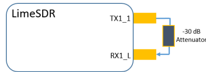
Figure 35: Setup to check the RX path of the LimeSDR with the generated pulses from the TX path.
