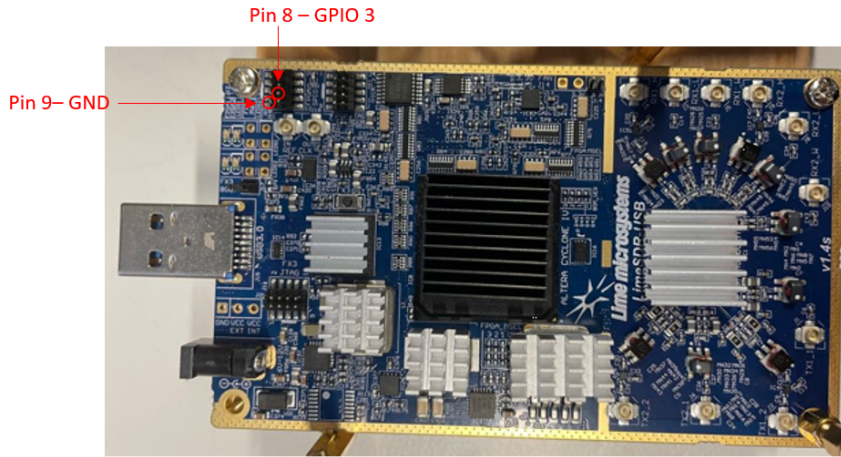
Figure 30: LimeSDR board with the GPIO Pin used marked in red.
