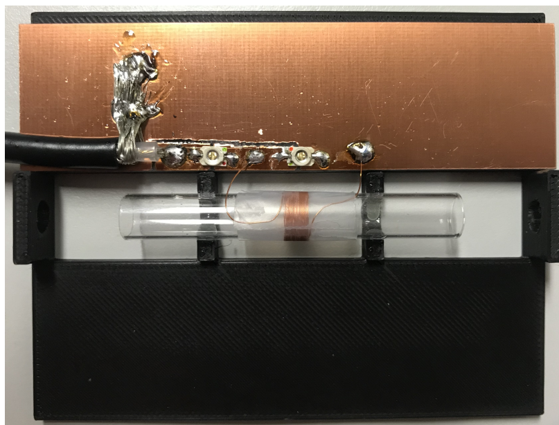
Figure 3.12: Probe holder and RF coil with tuning and matching capacitors The capacitors are tunable from 4.5 to 20 pF of make JZ200HV. The coil has a diameter of d = 7.5 mm, wire diameter D = 0.2 mm and n = 18 turns on a length of l = 4 mm. It has a measured inductance of L_{1\text{MHz}} = 2.7 \mu\text{H} and a resistance of R_{1\text{MHz}} = 0.63 \Omega . The body was 3D printed and the circuit cut by hand.
