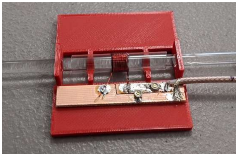
Figure 3.10: Manufacturer's probe holder and RF coil with tuning and matching capacitors The body was 3D printed and the circuit cut by hand.
